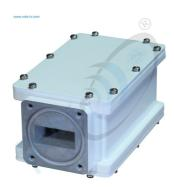
LNB-XPxx is a PLL LNB with single local oscillator and single output. LO instability  $\pm$  25 kHz, Gain 60dB, Noise figure 0.8 dB, Output power P1dB +5 dBm.
