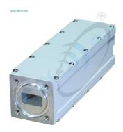
LNB-KuPxxD v1 is a PLL LNB with dual local oscillator and dual 750hm F-type output. LO instability  $\pm$  10 kHz, Gain 55dB, Noise figure 0.8 dB, Output power P1dB +6 dBm.
