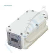
LNB-KuPxx v1 is a PLL LNB with single local oscillator and single 750hm F-type output. LO instability  $\pm$  25 kHz, Gain 60dB, Noise figure 0.9 dB, Output power P1dB +3 dBm.
