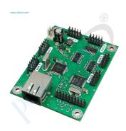
Control board 6ch is used for management and monitoring of various digital broadcasting equipment through TCP /  $\rm IP$
